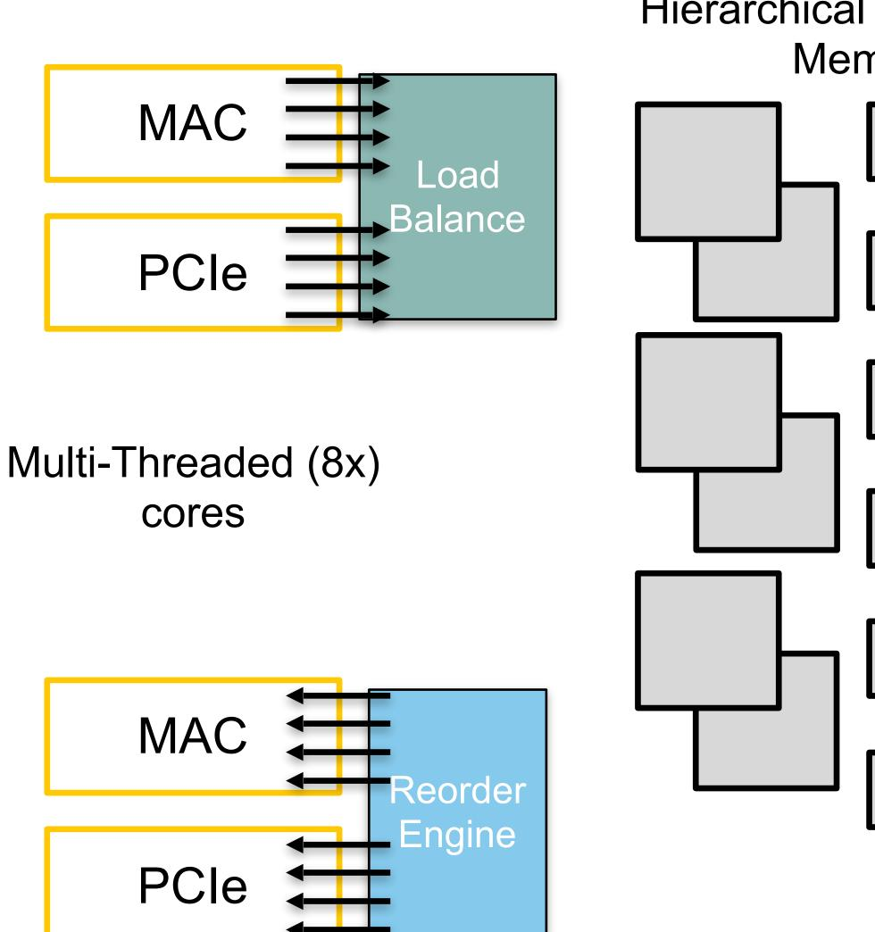
Reorder Engine is Key Feature due to the Many Multi-Threaded NPUs with specialized use of ~1000 simultaneous threads hardware offload
